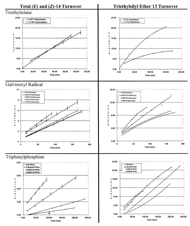
Fig. 2. Initial turnover rate studies for the reaction of ketone 9 with triethylsilane catalyzed by complex 2. The reaction additive is highlighted for each set of experiments.
